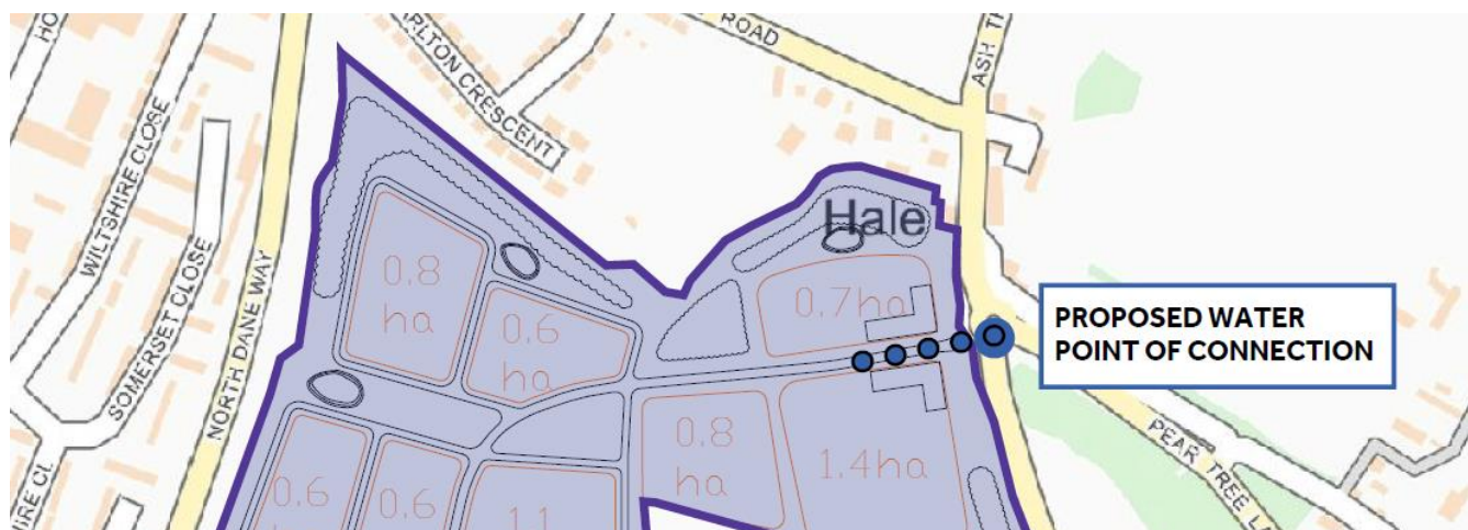
Figure 13 – Assumed potable water connection point
