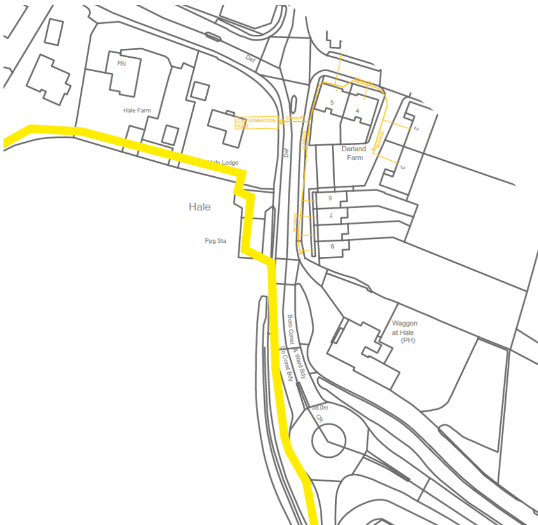
Figure 20 – GTC gas network adj. Capstone Road
