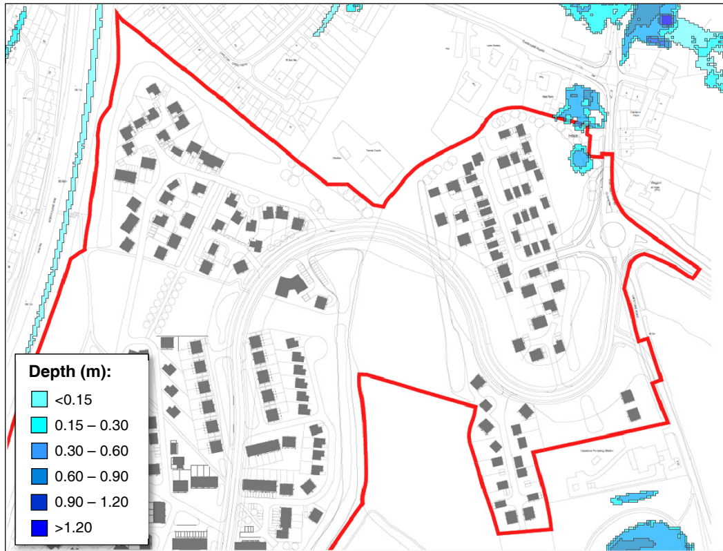
Figure 5.1 – Extract from the Environment Agency 'Risk of Flooding from Surface Water' Maps showing indicative flood depths for the 1 in 100 year extreme rainfall event (© Environment Agency).
