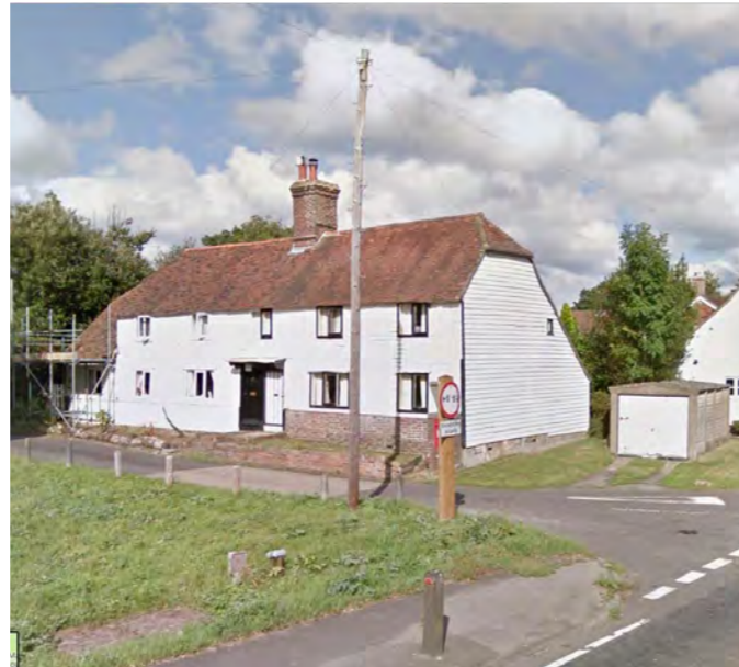
Asymmetric composition, half-hipped roof, full-height timber weatherboarding, mixed window types
