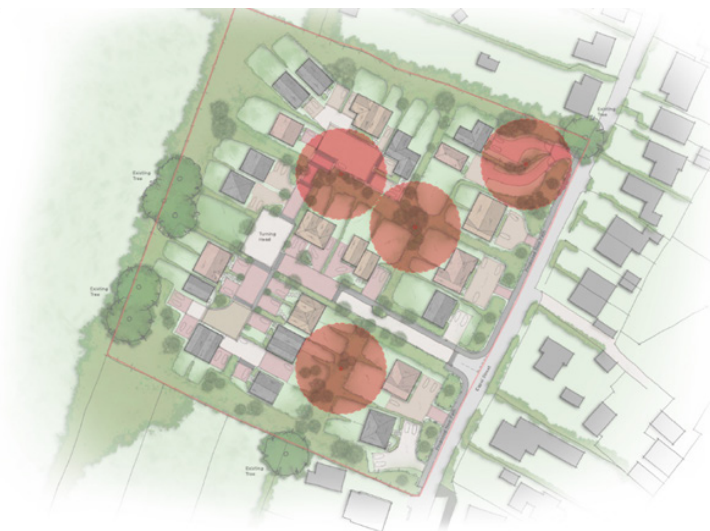
Figure 7. Locations of the four deep borehole soakaways.
