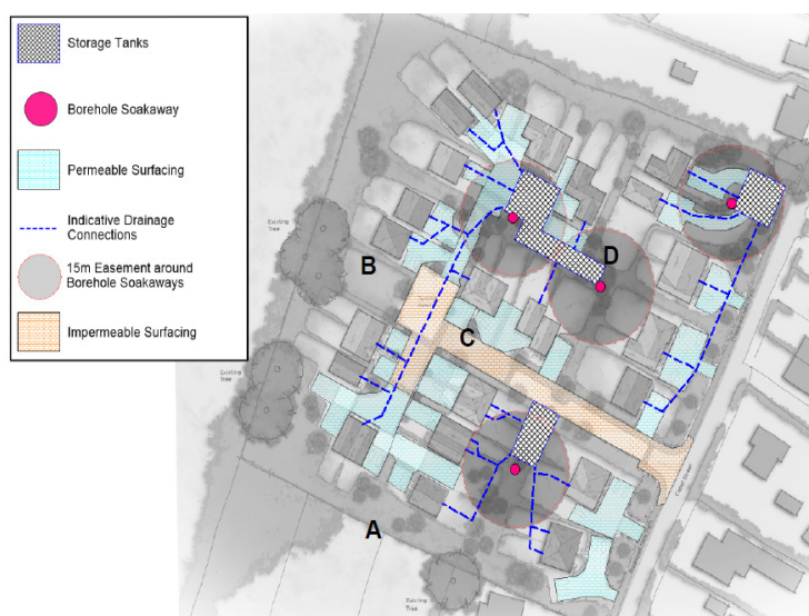
Figure 8. Layout showing the drainage strategy.
