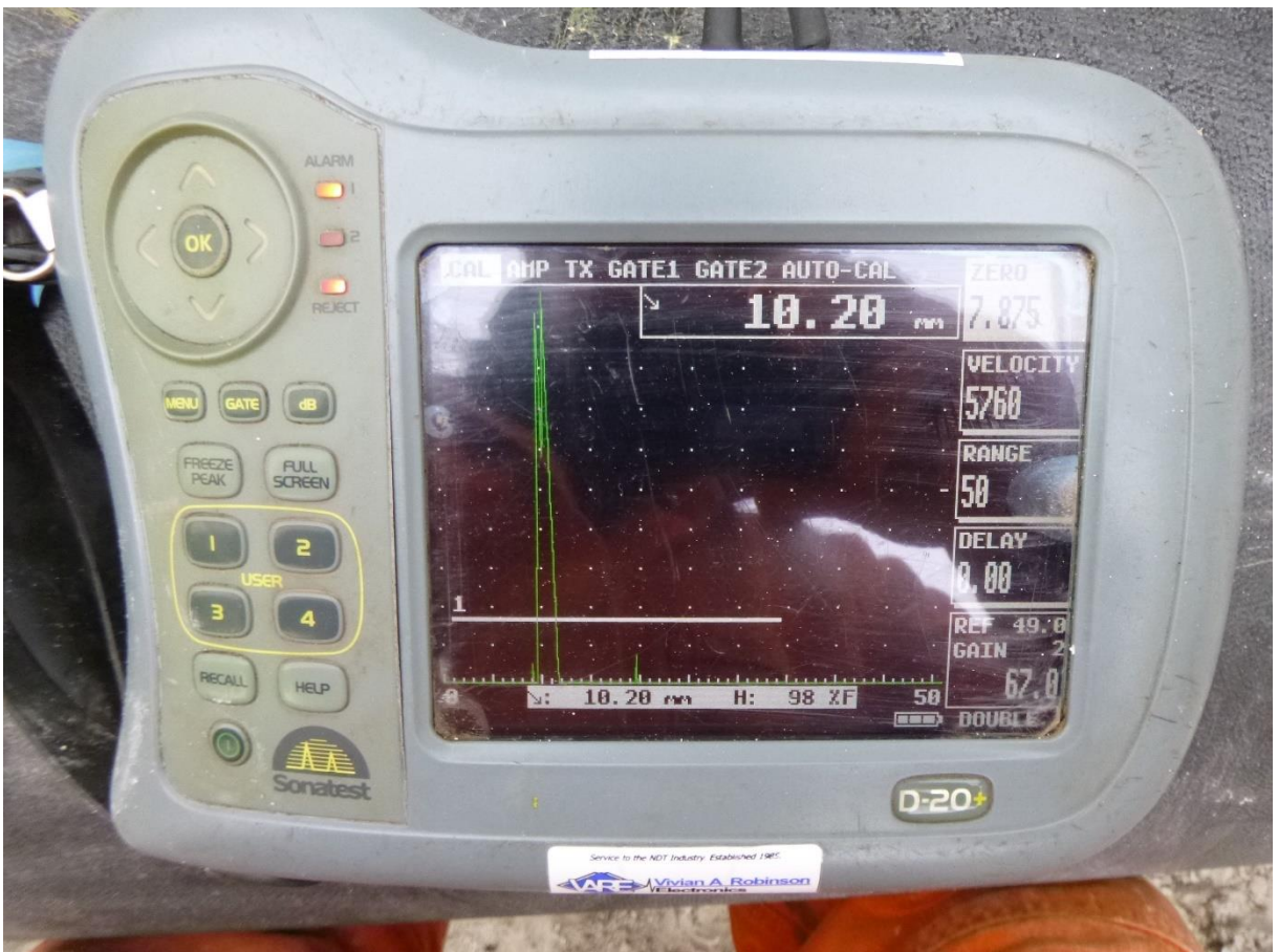
FIGURE A1.7 – UT PERFORMED ON MAIN
