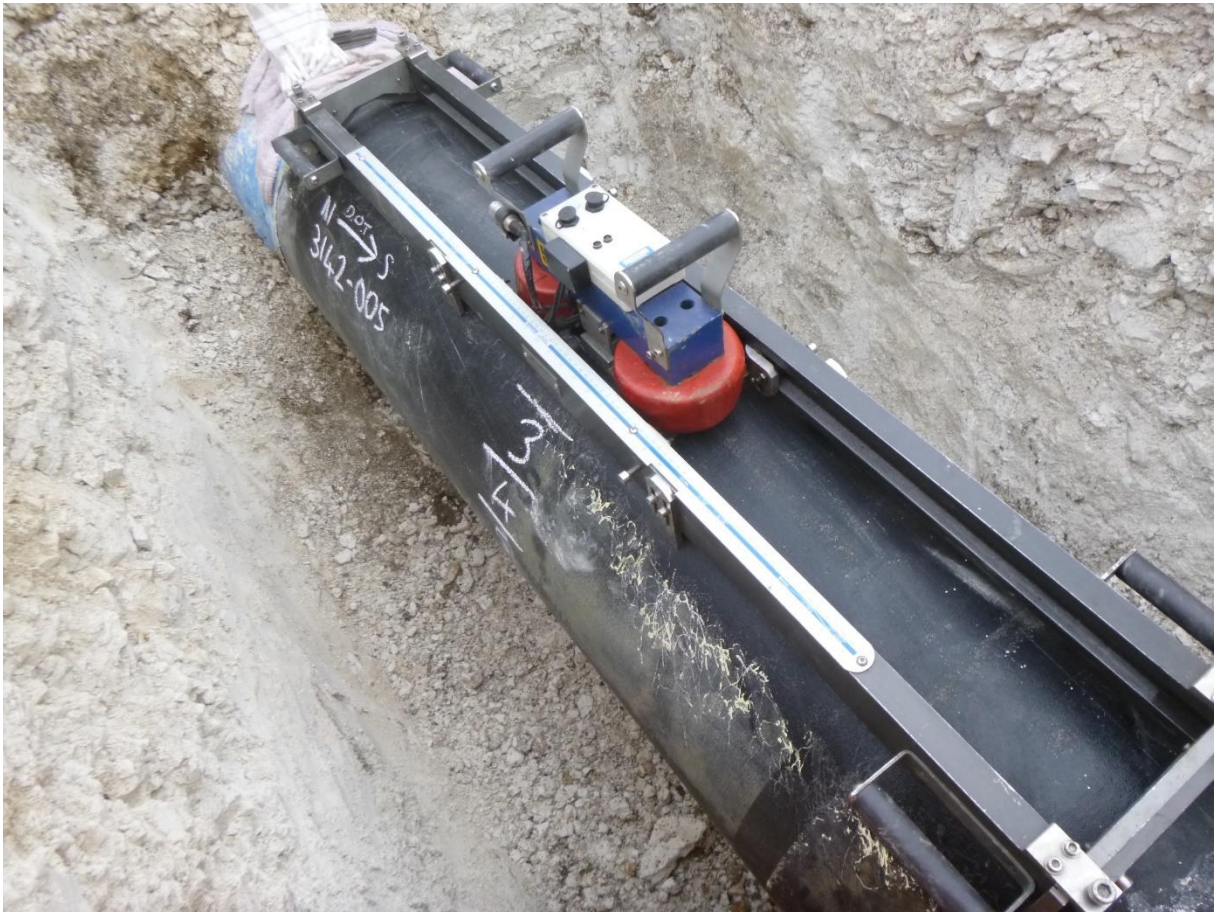
FIGURE A1.8 – MFL CARRIED OUT ON MAIN WITH SMARTCAT TOOL
