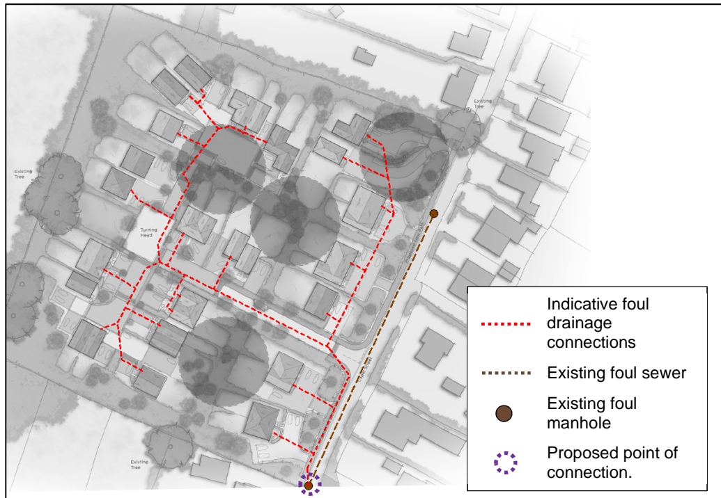
Figure 5.1 – Indicative foul drainage layout plan.
