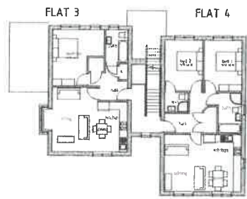
first floor plan FLATS 3 & 4 gross internal floor areas: flat 1, 705 sq m (70) flat 2, 705 sq m (70) flat 3, 576 sq m (50) flat 4, 795 sq m (70) (Minimum national described space standards in brackets) gross external floor areas: flat 1, 829 sq m (first circulation) flat 2, 821 sq m flat 3, 684 sq m flat 4, 821 sq m gross external floor area for both floors including shared circulation 243 sq m 195 sq m ground floor, 64 sq m first floor footprint 185 sq m
